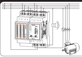
The PNM-31 voltage relay is applicable together with the LDM-30 voltage indicator. Three-phase system voltage is being measured in the relay circuit. The relay outputs cut OFF load power supply (e.g. the motor) in case of the preset voltage range exceeding. The voltage indicator enables continuous voltage visualization for the controlled circuit.
