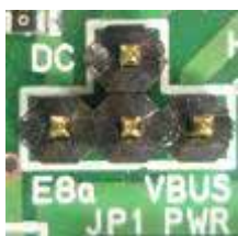
Figure 3 JP1 Main power supply switch
