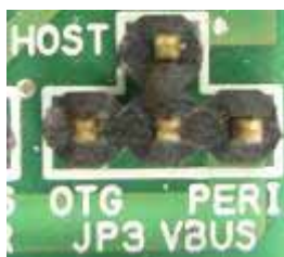
Figure 6 JP3 VBUS switch
