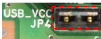
Power supply “ON” (Short) setting
