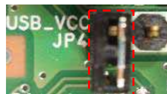
Power supply “OFF” (Open) setting
