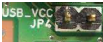
Figure 7 JP4 USB_VCC switch
