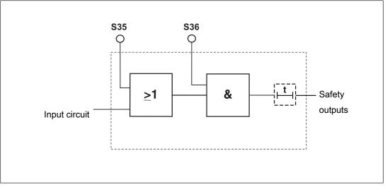
Logic inputs S35 and S36 from the PNOZ e4vp enable additional PNOZelog or PNOZmulti units to be logically AND/OR connected.
