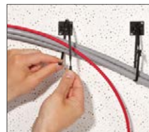
Without additional effort only Q-ties can be used for temporary and final cable bundling.
