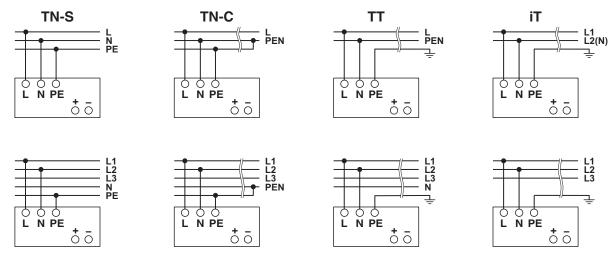
The connection for 100 V AC ... 240 V AC is established using the L, N, and P screw connections. The device can be connected to 1-phase AC networks or to two of the phase conductors of three-phase systems (TN, TT or IT systems in accordance with VDE 0100-300/IEC 60364-3) with nominal voltages of 100 V AC ... 240 V AC. The device also continues to work on short-term input voltages > 300 V AC.
