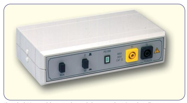
The Voltech PS1000 solid-state switch controls the turn-on of an AC supply to allow accurate measurement of the inrush current into an AC load. It is designed for use with Voltech power analyzers such as the PM100, PM300 or PM3000A.
