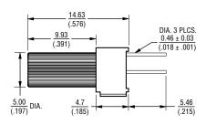
DIMENSIONS:  $\frac{\text{MM}}{(\text{INCHES})}$ TOLERANCES:  $\pm \frac{0.25}{(.010)}$  EXCEPT WHERE NOTED
