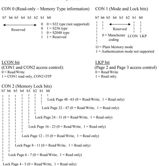
Note that CON2 (Memory Lock bits) are OTP (One-Time-Programmable) if LCON = 1 Note also that the "Reserved" bits must not be altered. Page 1 must be read first and the bits that can be changed masked on/off before writing back.
