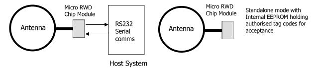
Remote mode (connected to a host computer or microcontroller) and Standalone mode.
