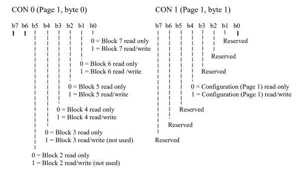
Note that these configuration bits are OTP. Once they are set to read-only the Hitag 1 transponder is hardware protected and they can never be changed.
