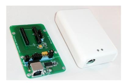
The Universal Socket board has the same basic footprint and mounting holes as the OEM-MICODE boards and has been designed to fit in the IBT plastic case.
