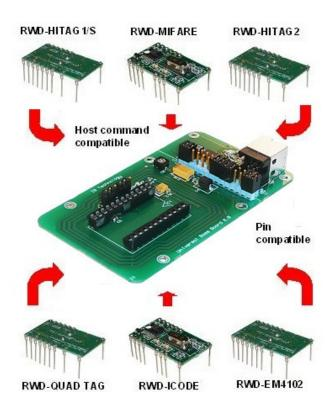
The Universal Socket board provides the antenna, and the serial-to-USB interface to the MicroRWD module. Specifically the board has a 24-pin DIP socket for the appropriate MicroRWD module to be plugged into, LEDS for visual status indication and selectable PCB and coil based antenna for 13.56MHz or 125kHz operation.
