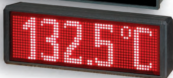
matryca LED array 56 x 16 wall housing 300 x 106 x 50mm, supply 24VDC
