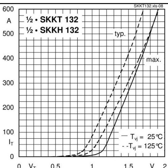
Fig. 7 On-state characteristics
