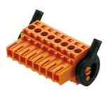
Female connectors with clamping yoke screw system for connecting conductors at 3.50 mm pitch. They include space for labelling and can be coded.
