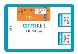
ULINKplus is a universal debug and trace adapter that enables test automation, software optimization for ultra-low-power applications, and isolation for debugging sensitive hardware systems. The compact enclosure allows usage in harsh environments and provides standard target connectors for JTAG, power measurement, and general purpose I/O.
