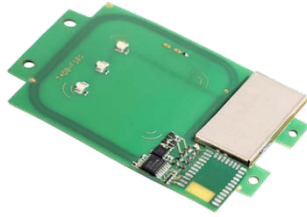
TWN4 MultiTech 2 HF PCB top view
