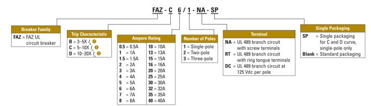
**1**  $I_n$  = Rated current for instantaneous trip characteristics.
