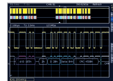
HEX decoded CAN bus signal
