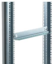
Equipment Guides help support rack-mounted equipment during installation. Guides mount between two pairs of rack angles. Slotted holes are provided for vertical or lateral adjustment. Furnished in pairs. Guides have plated finish. Mounting hardware included.
