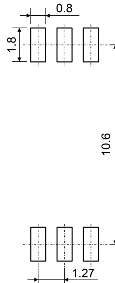
Fig. 15.2 Lead Forming Option (LF4)
