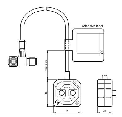
The unit can be switched from the V15 cable connection socket and the V15 plug connection on the sensor for the TEACH-IN procedure.
