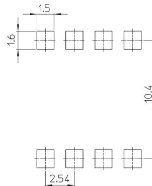
**Fig. 12.2 Lead forming and taping option (LF4), (TP4)**
