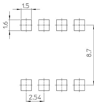
**Fig. 12.1 Lead forming and taping option (LF1), (TP1), (LF5), (TP5)**
