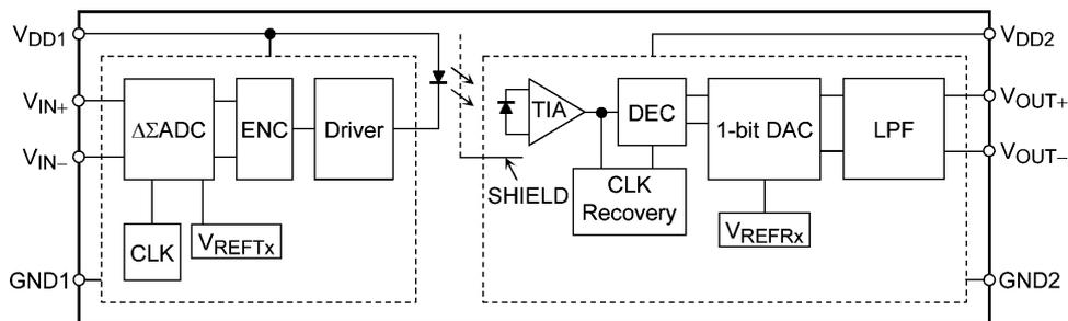
Note: A 0.1  $\mu$ F bypass capacitor must be connected between 1 and 4 pins and between 5 and 8 pins.
