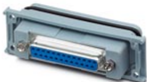
D-SUB panel mounting frame, shell size 3, with 25 signal contacts, socket, gender changer, shielded, IP67 degree of protection
