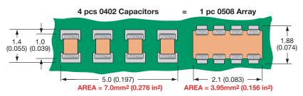
The 0508 4-element capacitor array gives a PCB space saving of over 40% vs four 0402 discretes and over 70% vs four 0603 discrete capacitors.
