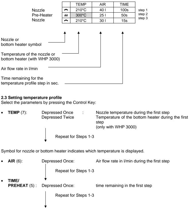
The active value is marked on the display and can be changed using the **UP / DOWN** (2) / (3) Control Keys. Keeping the Control Key depressed, rapidly changes the value.
