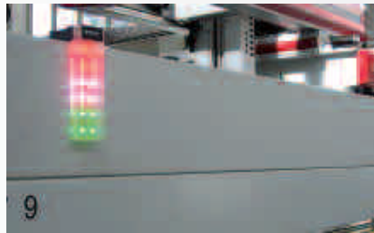
Tier-by-tier illumination of the lighting body
