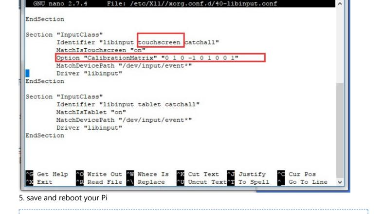
After completing these steps. The LCD could rotate 90 degree both display and touch.
