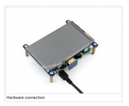
You can enable the touch in two ways: Method 1. install driver to your Raspbian/Ubuntu Mate OS. Method 2. use the Ready-to-use image file of which LCD driver was pre-installed.
