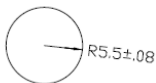
Recommended panel hole cutout (mm)
