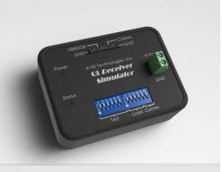
The Qi Medium Power FOD Receiver is a 15W receiver that can be used to test the operation and FOD performance of Qi wireless transmitters. DIP switches on top of the FOD Receiver are used to program received power offsets and to change internal loads.
