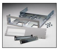
**4288-9:** Mounts 2U-high instruments in 3U-high rack space. 3U (5.25 in.) high. For use with: Series 2000, 2182A, Series 2300, 2700, 2701, 6220, 6221, 6485, 6487, 6514, 6517B, 7001
