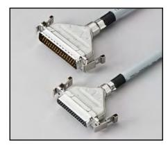
**Model 2000-MTCD-2 Cable Assembly:** 2-meter cable with a 44-pin connector on one end that is designed to mate with the 2000-SCAN-20 scanner card. The other end is equipped with a 50-pin D-sub male connector.
