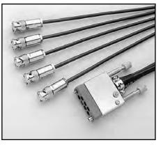
**Model 7153-TRX:** 2m (6.6 ft) low noise cable assembly with M-series connector at one end for row or column connections to the 7153, and five 3-slot male triax connectors at the other end. Two 7153-TRX cable assemblies are required to make all connections to the 7153 card.
