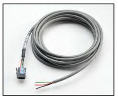
**Model 2290-INT-CABLE:** Safety interlock cable, 3.05m (10 ft). 3-conductor cable with 3-pin connector on one end and unterminated wires on the other end.
