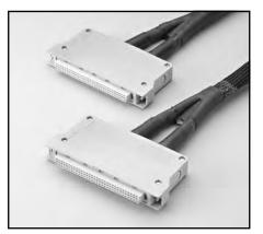
**Model 7036-MTC-2:** 2m (6.6 ft) mass terminated cable assembly for connection to 7036. The cable has 45 pairs with outer shield. The cable is terminated at each end with 96-pin female DIN connectors with strain relief.
