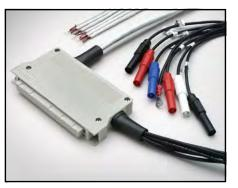
**Model 7019C-MTCI-2 6-wire Kelvin Extender and Instrument Cable:** Used with Model 7019-C 6-Wire Ohms Matrix Card and a SourceMeter SMU instrument. The SourceMeter cables are 0.6m (2 ft) long and the DUT cables are 2m (6.6 ft) long. The cable set is used in a basic system to test a resistor network.
