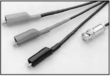
Model 237-ALG-\*: Low noise triax cable (SC-22) terminated with a 3-slot male triax connector on one end and 3 alligator clips on the other. 237-ALG-2 2m (6.6 ft) length 237-ALG-15 15m (50 ft) length
