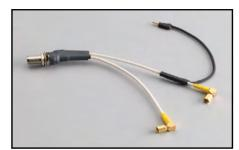
**Model 4200-PRB-C:** SMA to SSMC Y adapter cable with local ground that connects the 4200-PIV package to DC probe manipulators. The cable is terminated at one end with a single female SMA. The other end splits into two gold SSMC plugs (female connectors) and a black wire with integrated connector, which is used to connect to the shield of another Model 4200-PRB-C cable.
