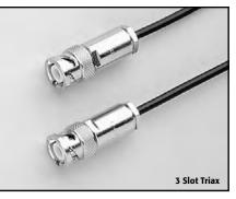
**Model 7078-TRX-GIN 3-slot Triax Cable:** 0.15m (6 inch), 3-slot, low-noise, guarded triax cable that minimizes leakage current and input capacitance when used with the Model 6430 Remote PreAmp (lower noise than 1 foot or longer versions).
