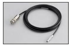
**Model 4200-MTRX-\*:** Ultra low noise SMU triax cable is terminated with a miniature male triax connector on one end and a standard 3-slot male triax connector on the other end. This cable connects a Model 4200-SMU or 4210-SMU source measurement unit installed in a Model 4200-SCS to a test fixture. (4200-MTRX-\* cables are intended only for connection to an SMU that does not have a 4200-PA PreAmp installed.)
