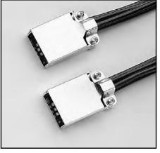
Model 7152-MTC-\*: Five low noise triax cables terminated in 6-position M-series coax connector blocks. Provides quick connection between 7152 matrix cards and is compatible with Model 7152-MTR connector. Also available in 3m (10 ft) length for connection between the matrix and the device under test. 7152-MTC-2 0.6m (2 ft) 7152-MTC-10 3.0m (10 ft)
