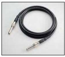
**Model 2290-10-SHV:** 3m (10 ft) of RG-213/U coaxial cable terminated with a SHV male connector on both ends. Maximum operating voltage is 10,000Vrms.
