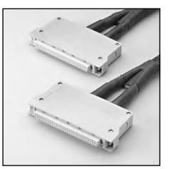
**Model 7011-MTC-x:** Mass terminated cable assembly for connection to 7011-C and other switching cards. The cable has 45 pairs with outer shield. The cable is terminated at each end with 96-pin female DIN connectors with strain relief. **7011-MTC-1** 1m (3.3 ft)
