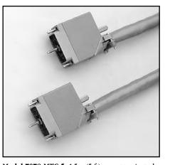
**Model 7078-MTC-5:** 1.5m (5 ft) mass terminated cable for connection to column inputs (7071 and 7071-4). Also used for matrix expansion (7071, 7071-4, or 7074). The cable has 12 sets of shielded twisted pair wires for isolation of critical circuits and noise rejection in the system. The cable is terminated at each end in a 38-pin connector block with strain relief. **Model 7078-MTC-20** can be used as is or cut in half to make two 10 ft cables.
