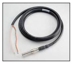
**Model 2290-10-SHVUC:** 3m (10 ft) of RG-213/U coaxial cable terminated with a SHV male connector on one end and unterminated cable on the other end. Maximum operating voltage is 10,000Vrms.
