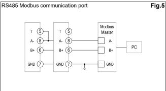
Additional instruments with RS485 are connected in parallel. The serial output must only be terminated on the last network device connecting terminals A- and T. For connections longer than 1000 m use a signal repeater. Maximum 247 transceivers on the same bus.
