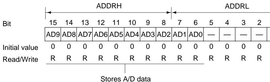
Correspondence between analog input channels and ADDR registers
