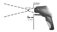
If a measurement distance > 250 mm, switch over to far field measurement.
