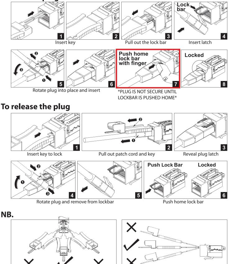
Key must be inserted perpendicular to the socket
