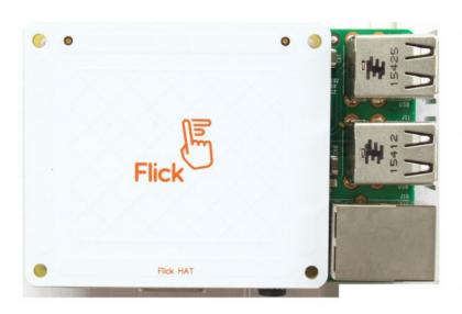
**Step 5** - Screw the last 4 plastic bolts to hold the Flick HAT in place.
