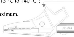
Barrier. Keep behind this barrier to operate safely the clip while connecting to hazardous live voltages (more than 33 V AC and 70 V DC).
