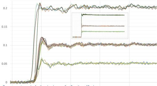
PicoConnect passive probe family pulse shapes – first 2 ns (inset 17 ns)
