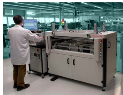
Electrical final test
