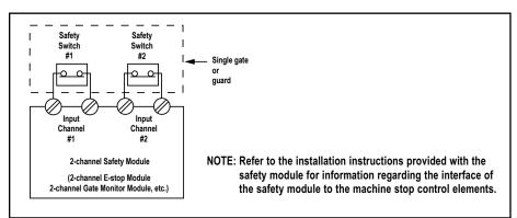
Figure 2. Connect two redundant safety switches per interlock guard to an appropriate 2-channel input safety module.
