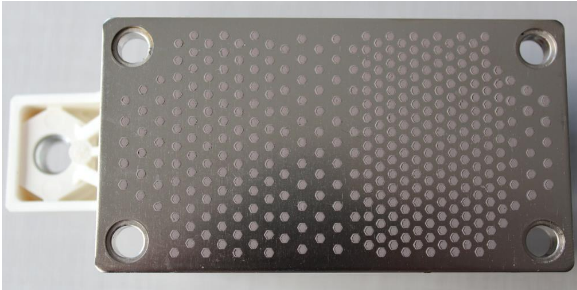
Figure 5: Module printed with TIM (Thermal Interface Material)
