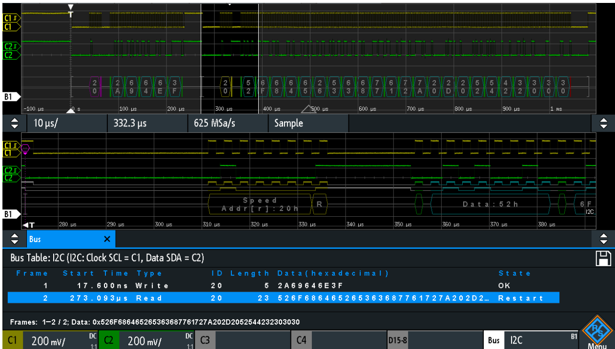
Figure 12-14: Decoded I2C signal with applied label list and zoom on second frame
