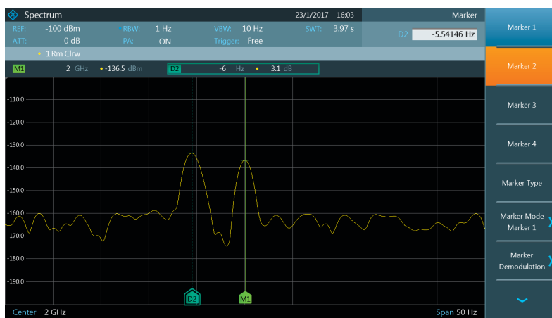
R&S®FPC-B22: high sensitivity with 1 Hz resolution bandwidth.
