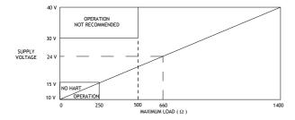
[(Vsupply -10)/21.5]  $K\Omega$ , 250  $\Omega$ Max Output Load
