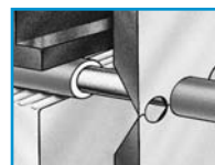
Knife-type stripping blades have form-ground holes which penetrate the insulation like a knife, giving a clean insulation cut.
