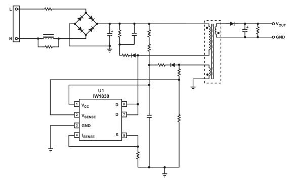
Figure 3.1 : iW1830 Typical Application Circuit
