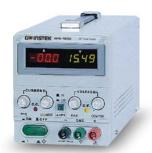
The SPS-Series are single output, 360W, switching DC power supply. OVP protects the SPS-Series and their load from unexpected conditions. High regulation is maintained at 0.01%. Remote sensing adds extra level of precision by compensating cable losses between loads. Turning the output On/Off from external device is available through Remote control terminals. The GPS-Series are an ideal solution for power-efficient bench-top or portable applications requiring high regulation.
