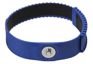
The Wristband 4600 Series consists of an insulative exterior with conductive interior and metal male snap available in 4mm. Made of thermoplastic material, the Wristband 4600 Series is lightweight, low profile and safely makes contact with human skin, assuring employee acceptance while helping to ensure ease of use. The "zipper" style latching mechanism easily adjusts to most wrist sizes.
