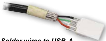
Solder wires to USB-A Insert
