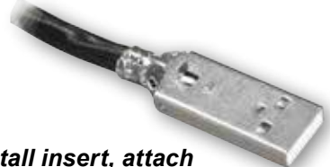
Install insert, attach lid, and crimp shield
