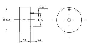
Dimensions : Millimetres Tolerance: ±0.5mm
